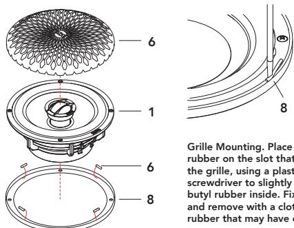
Grille Mounting. Place the butyl rubber on the slot that houses the grille, using a plastic flat screwdriver to slightly push the butyl rubber inside. Fix the grille and remove with a cloth any butyl rubber that may have come out.
